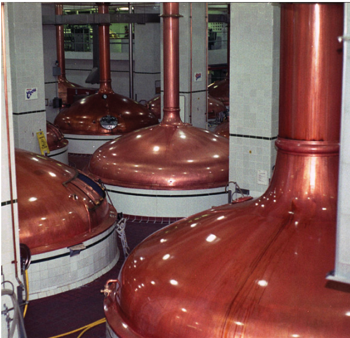
Figure 6.9 An oxide of carbon is removed from these fermentation tanks through the large copper pipes at the top. By: Rice University Openstax CC BY NC SA
