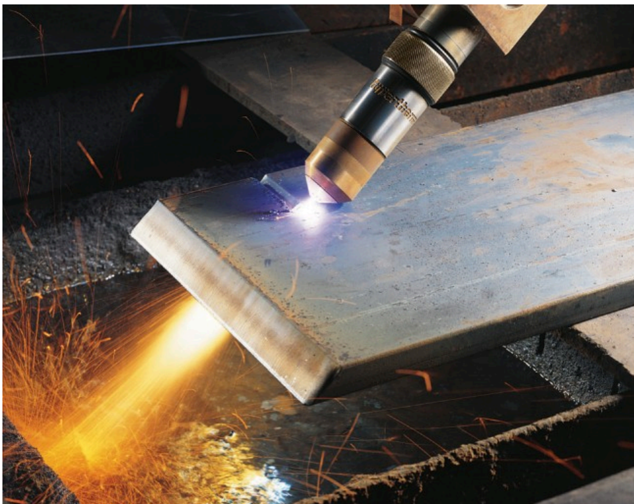
Figure 1.7 Torch Cutting Closeup. A plasma torch can be used to cut metal. Wikimedia Commons. By: Hypertherm Wikimedia Commons CC BY NC SA
