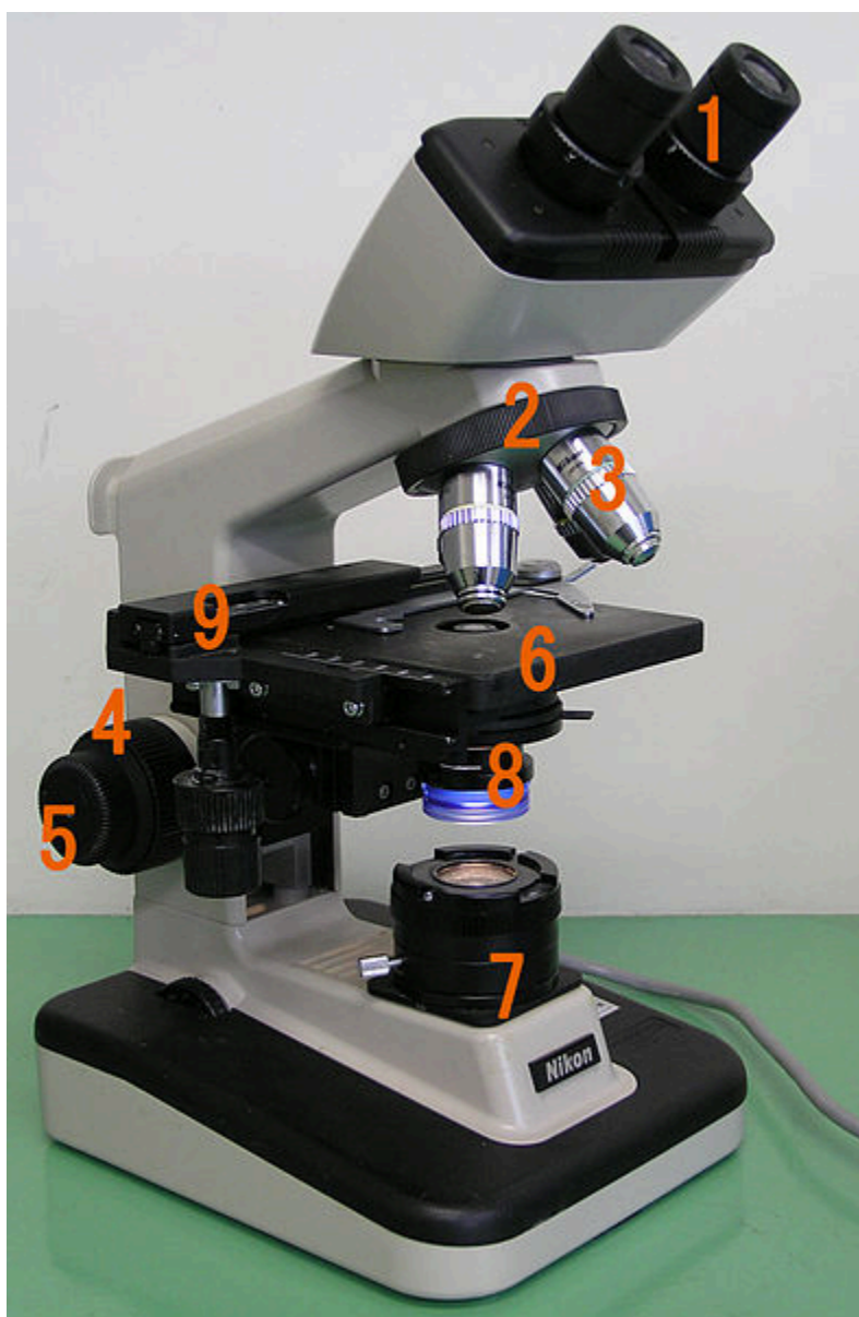
Figure 2.1: The parts of the microscope. By GcG(jawp) and under the Public Domain. https://commons.wikimedia.org/wiki/File%3AOptical_microscope_nikon_alphaphot.jpg
