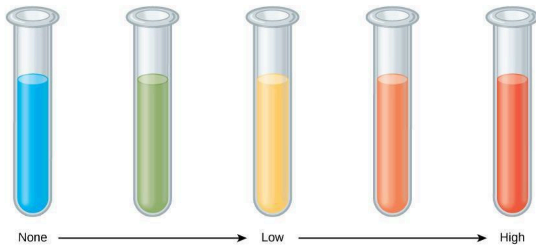
Figure 3.6: Benedict's test results for glucose concentration.
