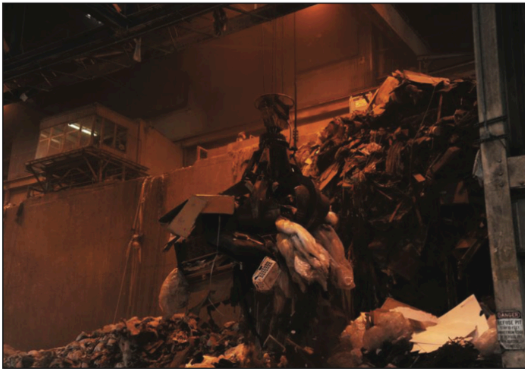
Figure 13.9 The “Claw” moving plant waste and rubbish to the incinerator; Author | Senior Airman Sam Fogleman; Source | U.S. Air Force; License | Public Domain.
