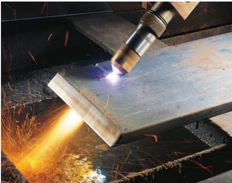
Fig. 4.3 A plasma torch can be used to cut metal.
