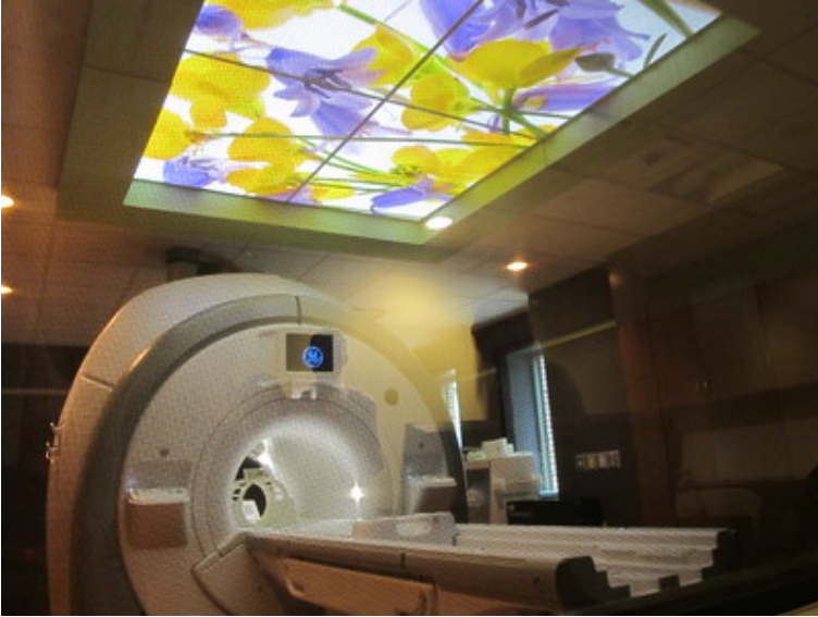
Fig. 10.7 Instrument for magnetic resonance imaging (MRI). The device uses a superconducting cylindrical coil for the main magnetic field. The patient goes into this “tunnel” on the gurney.
