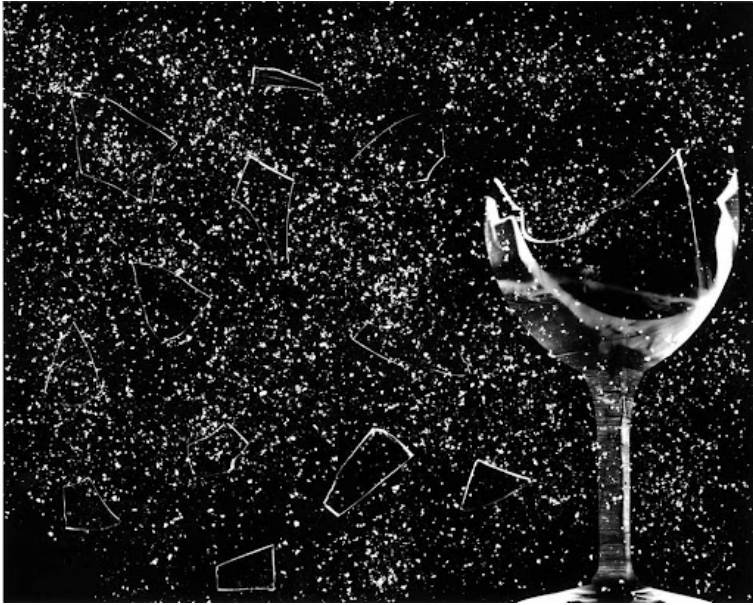
Fig. 5.23 This glass has been shattered by a high-intensity sound wave of the same frequency as the resonant frequency of the glass. While the sound is not visible, the effects of the sound prove its existence.
