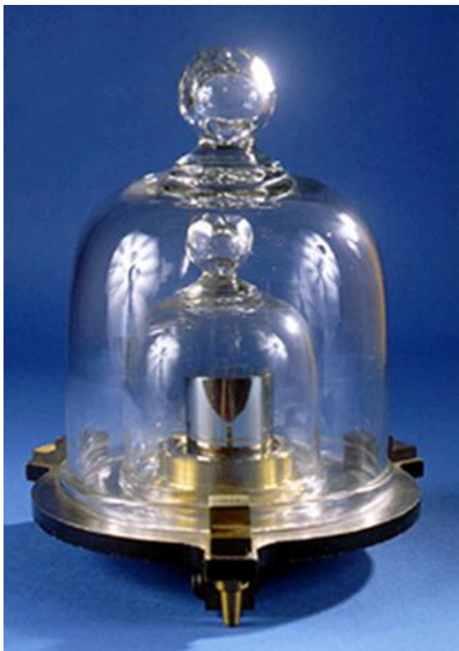
Fig. 1.4 This replica prototype kilogram (as previously defined) is housed at the National Institute of Standards and Technology (NIST) in Maryland.
