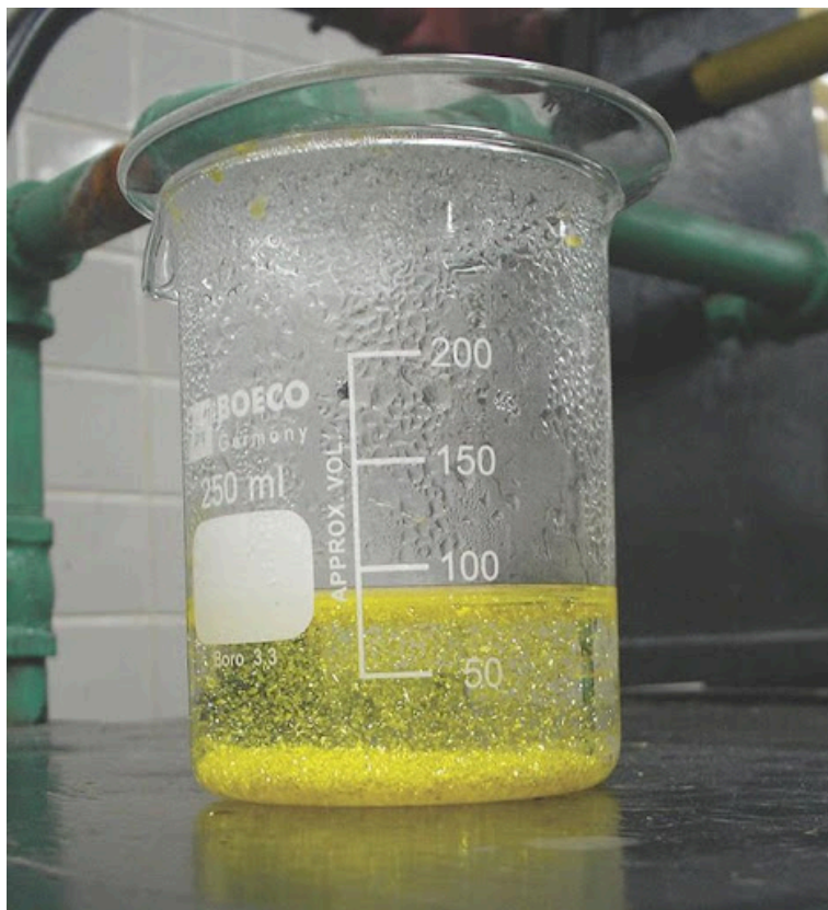
Fig. 4.7 A precipitate of \text{PbI}_2 forms when solutions containing \text{Pb}^{2+} and \text{I}^- are mixed.
