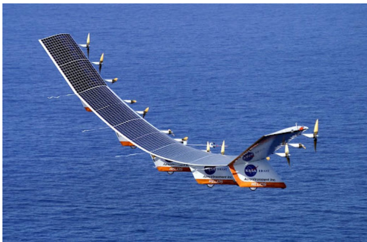
Fig. 8.5 Solar energy is converted into electrical energy by solar cells, which are used to run a motor in this solar-power aircraft.
