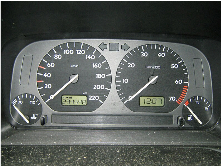
Fig. 9.16 The fuel and temperature gauges (far right and far left, respectively) in this 1996 Volkswagen are voltmeters that register the voltage output of “sender” units, which are hopefully proportional to the amount of gasoline in the tank and the engine temperature.
