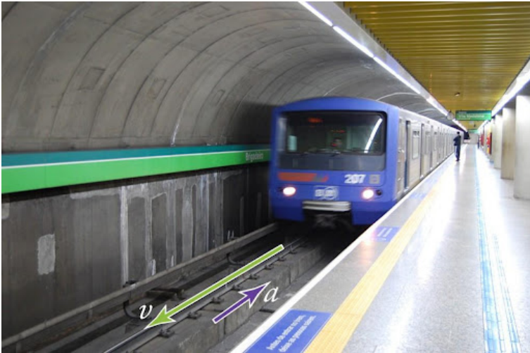
Fig. 2.9 A subway train in Sao Paulo, Brazil, decelerates as it comes into a station. It is accelerating in a direction opposite to its direction of motion.
